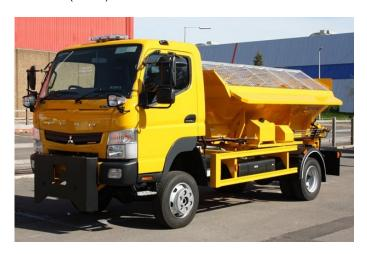
Side guards are fitted to reduce the likelihood of injury to 'unprotected road users' like pedestrians, cyclists and motorcyclists when struck by a vehicle travelling in a forward direction. They are fitted to deflect and to stop people falling underneath the sides of the vehicle and being caught underneath the wheels.
