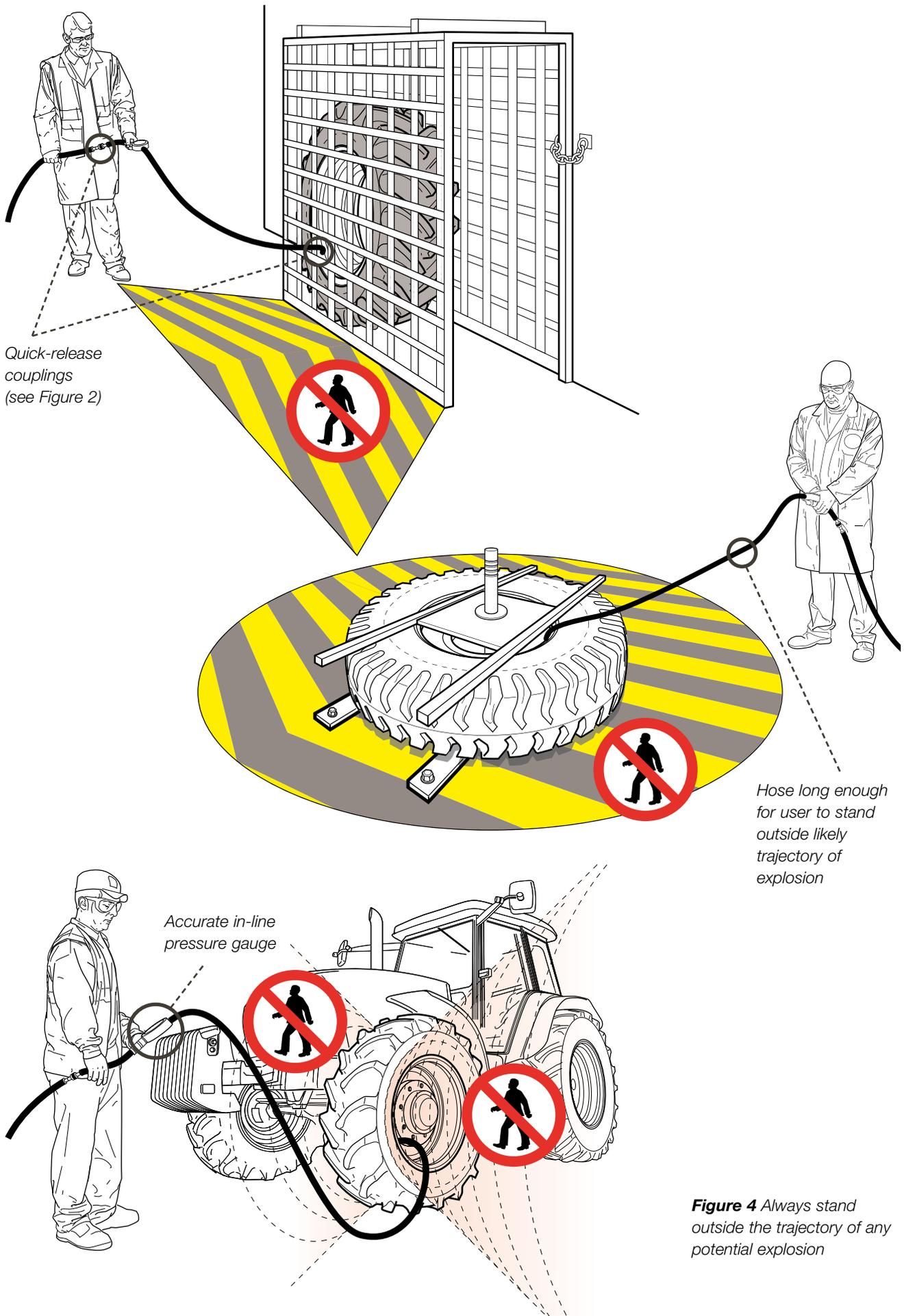
**Figure 4** Always stand outside the trajectory of any potential explosion
