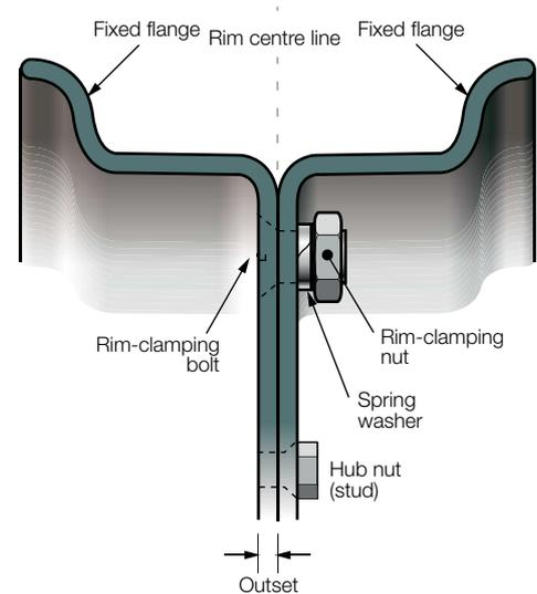
**Figure 9** Cross-section of a divided wheel
