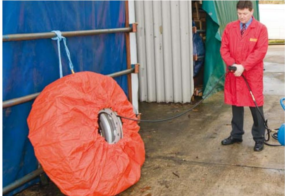
**Figure 5** A bag-type restraint
